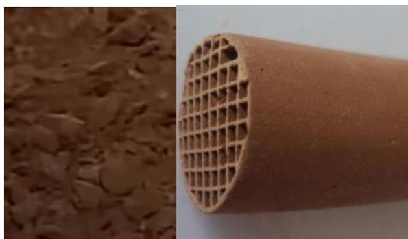
Photos of Argan fruit shells as precursor for supercondensator electrodes and honeycomb monolith extruded using local clay.
