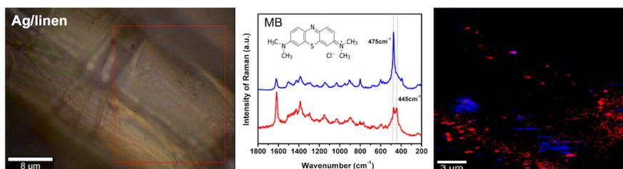
**Figure 1:** Optical photograph (right) and combined Raman image (left) using two different Raman spectra of MB ( $10^{-4}$  M) adsorbed on Ag/linen composite; chemical structure of MB and Raman spectra of MB species used for the combined Raman image (633 nm excitation laser source) (middle);
